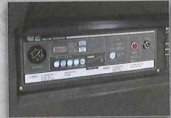
1 | Keyed Start and Digital Monitor with Auto Idle Mode
